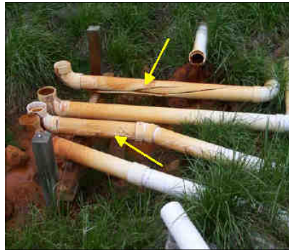
Center: Freezing temperatures resulted in broken pipes (highlighted by arrows).
